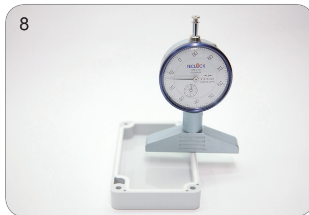
Check the depth and make sure the adhesive installation is OK
