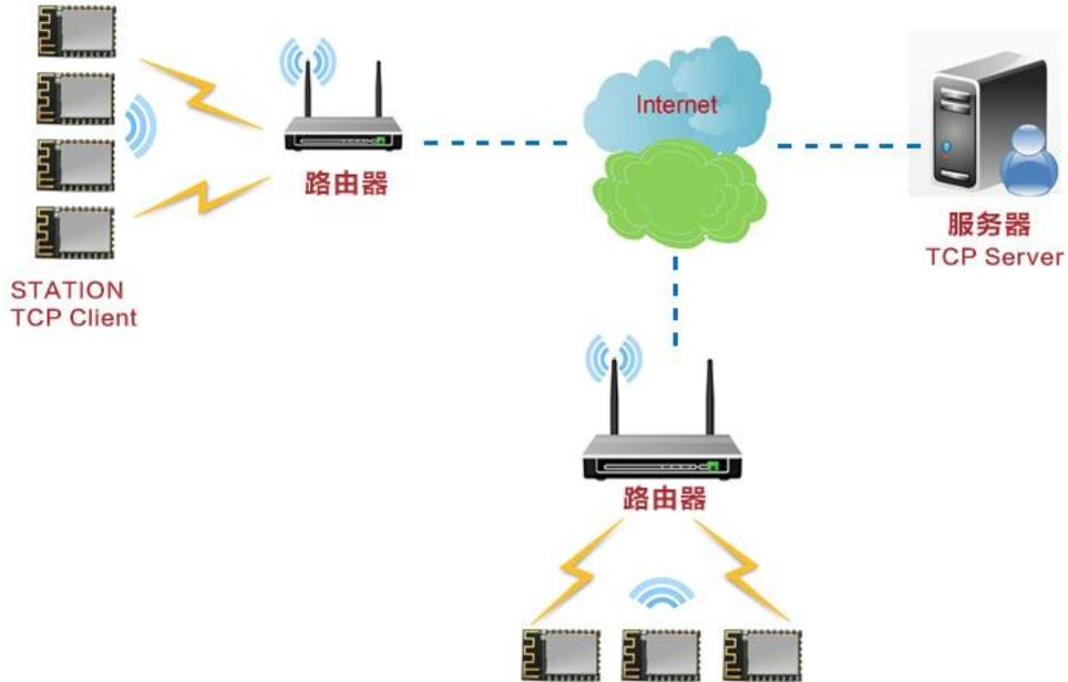
**Module build TCP Client to connect with wi-fi device when works at STATION mode**
