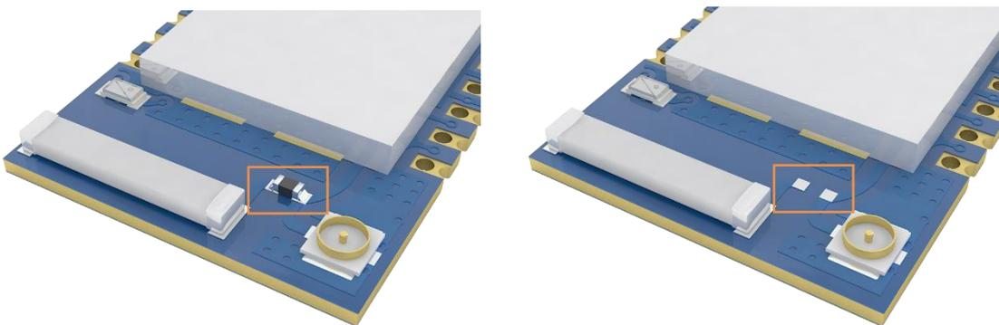
The default 0R resistor is soldered as shown above (left), and the antenna interface is ceramic antenna. If you need to change the antenna interface mode to IPEX, please change the 0R resistor to the above (right).
