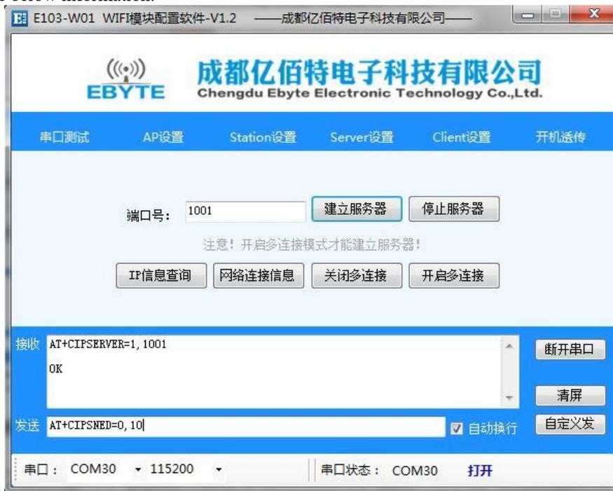
**【PC connected with TCP server of module to transmit data】 :**
