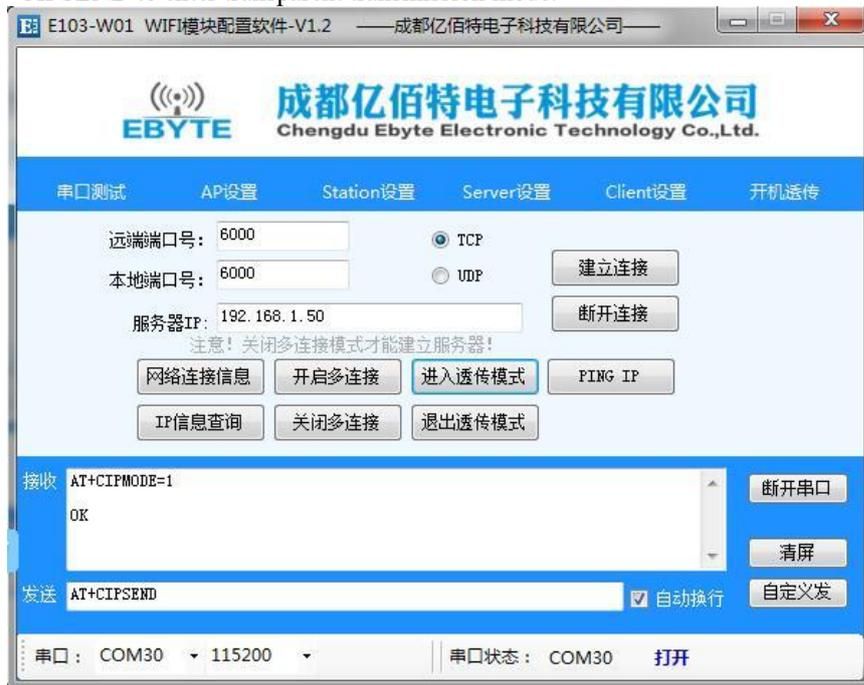
Notes: module no longer receive AT command, transmit the data from UART to server directly.
