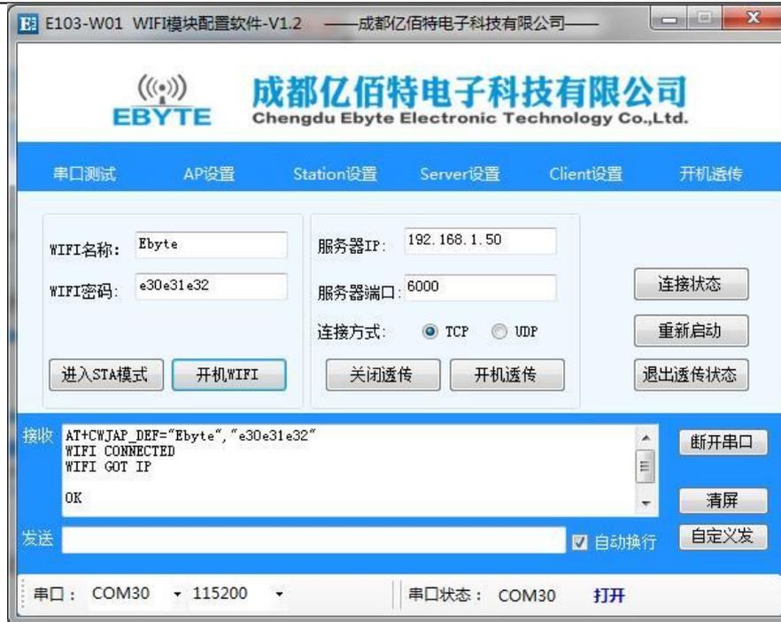
Input server IP address, port number, and choose TCP mode, then click “transparent transmission on power-up”, see below interface means configuration is done
