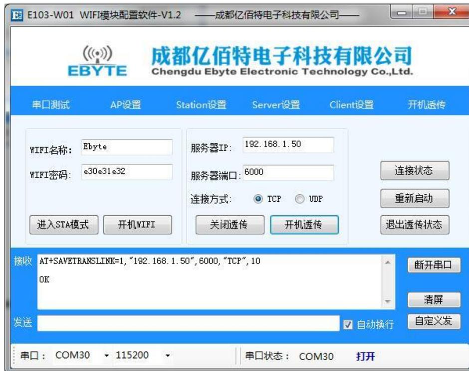
After click “re-start” or re-power the module, it will connect to the router and address automatically and the connection status can be judged by wi-fi indicator (GPIO2).
