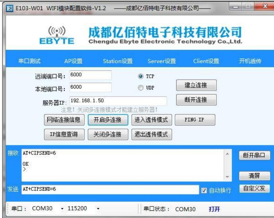
After “>” symbol shows, transmit data “123456”, user can see the TCP server receive data "123456". Data communication completed..
