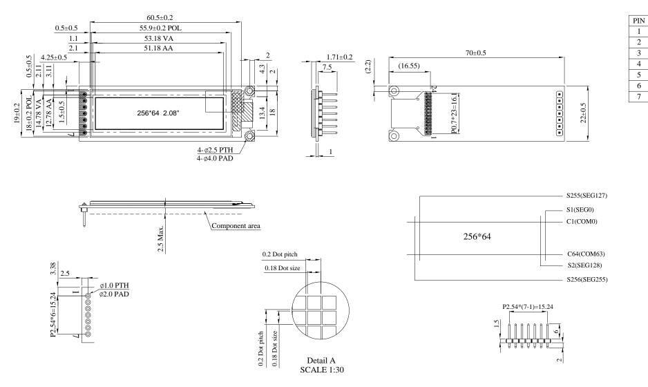
The non-specified tolerance of dimension is  $\pm 0.3 \mbox{ mm}$  .
