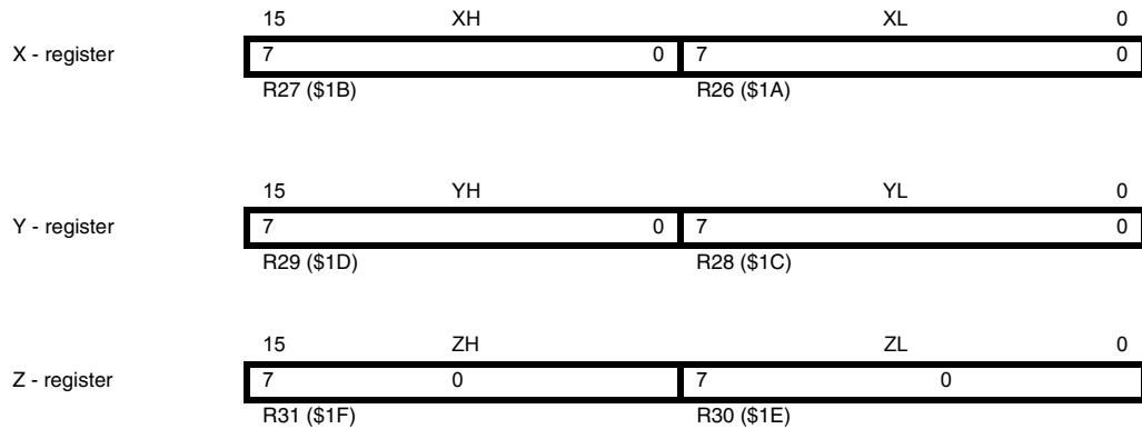
Figure 6-3. The X-, Y-, and Z-registers
