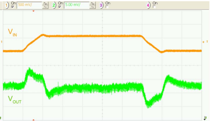
Figure 21. Line Transient 3.3V_{IN} to 3.9V_{IN} , 250mA Load, 10\mu s/div.
