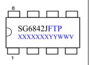
F: L = OTP Latch, C = OTP auto-recovery T: D = DIP, S = SOP P: Z = Lead Free + ROHS Compatible Null=regular package XXXXXXX: Wafer Lot YY: Year; WW: Week V: Assembly Location
