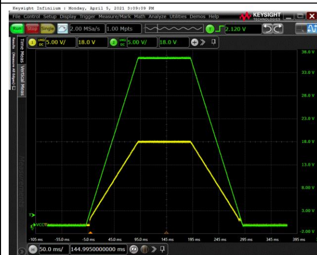
Figure 21. 100 ms, 0 V to 36 V Power on and off Time
