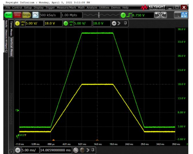
Figure 20. 10 ms, 3 V to 36 V Power on and off Time
