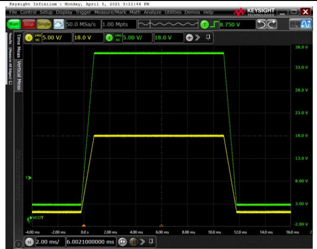
Figure 18. 1 ms, 3 V to 36 V Power on and off Time
