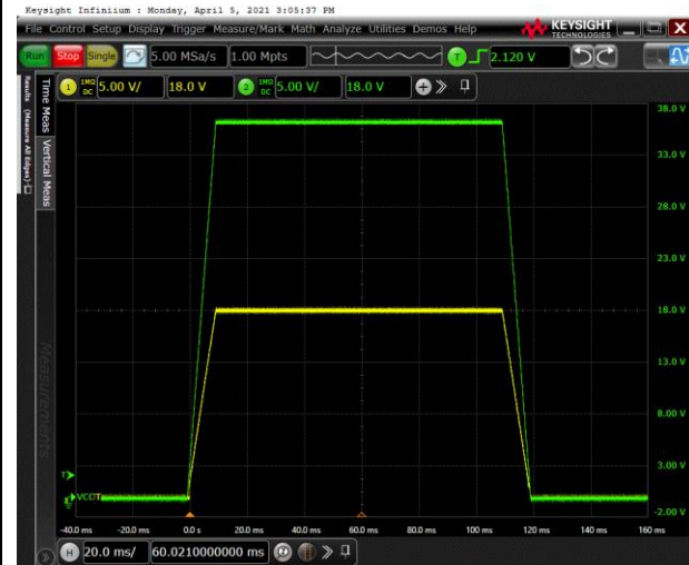
Figure 19. 10 ms, 0 V to 36 V Power on and off Time
