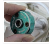
The palm ratchet for easy operation in limited areas
