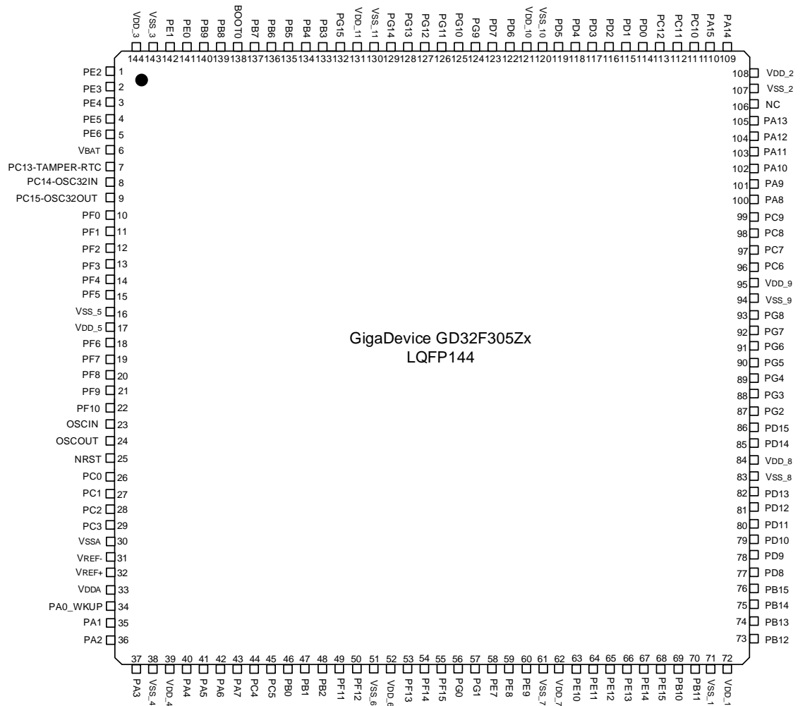
Figure 2-2. GD32F305Zx LQFP144 pinouts
