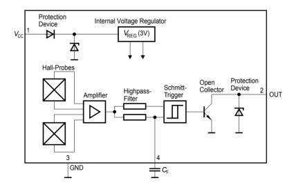
Figure 1. Functional Block Diagram of AH4921
