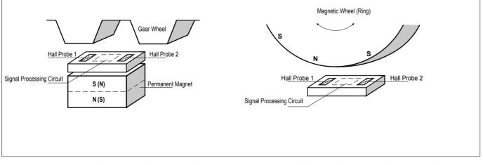
Figure 2. AH4921, with Ferromagnetic Toothed Wheel or Magenetic Wheel (Ring)
