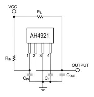
$$\begin{split} & C_F = 470 nF \ , \ R_L = 2k \ \Omega \\ & R_{IN} = 10 \ \Omega \ , \ R_{IN} \ is \ optinal; \\ & C_{IN} = 4.7 nF \ , \ C_{IN} \ is \ optinal; \\ & C_{OUT} = 4.7 nF \ , \ C_{OUT} \ is \ optinal; \end{split}$$
