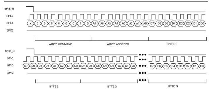
Figure 17. SPI Multiple Write
