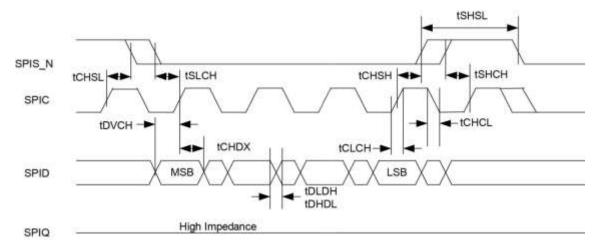
Figure 29. SPI Input Timing
