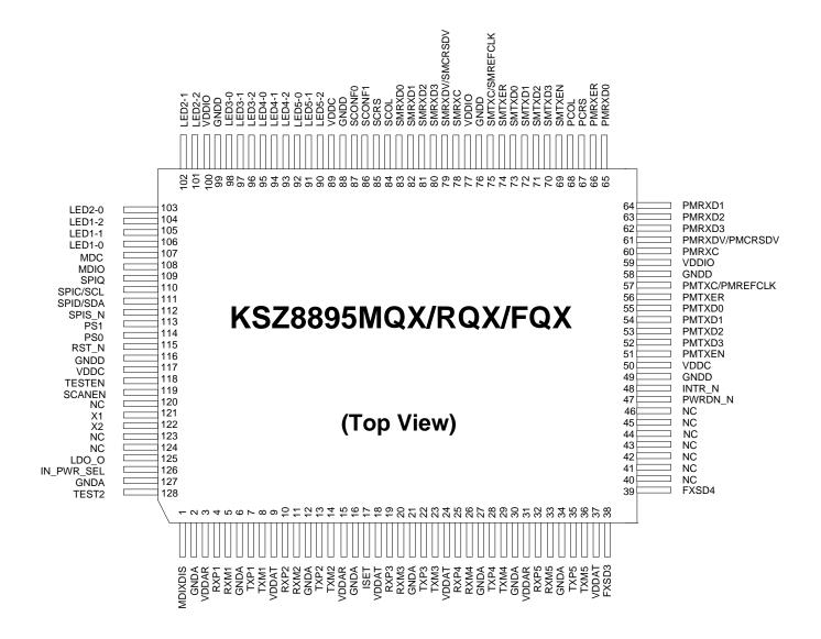
128-Pin PQFP Pin Configuration
