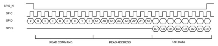
Figure 16. SPI Read Data Cycle
