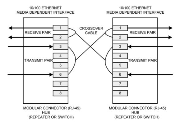
Figure 6. Typical Crossover Cable Connection
