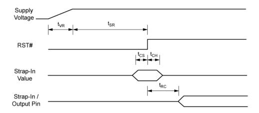
Figure 33. Reset Timing
