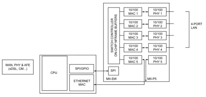
Figure 2. Integrated Broadband Router
