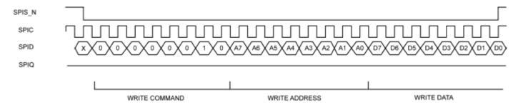
Figure 15. SPI Write Data Cycle
