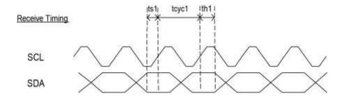
Figure 19. EEPROM Interface Input Receive Timing Diagram
