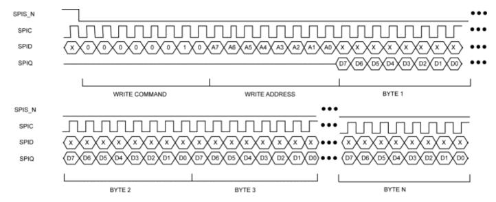
Figure 18. SPI Multiple Read
