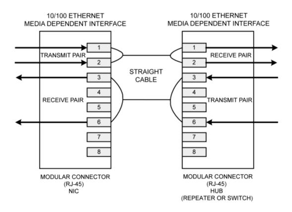
Figure 5. Typical Straight Cable Connection
