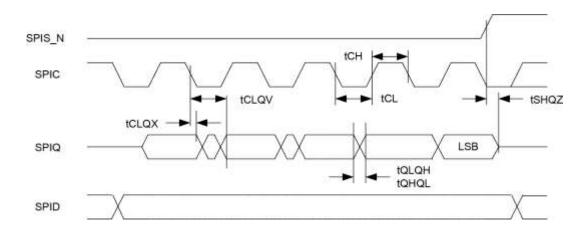
Figure 30. SPI Output Timing
