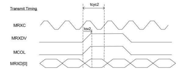
Figure 22. SNI Output Timing
