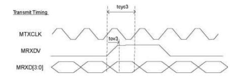
Figure 24. MAC Mode MII Timing – Data Transmitted from MII
