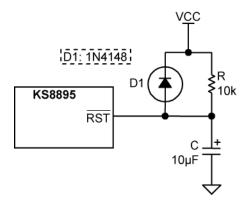
Figure 34. Recommended Reset Circuit
