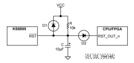
Figure 35. Recommended Circuit for Interfacing with CPU/FPGA Reset
