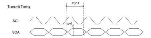
Figure 20. EEPROM Interface Output Transmit Timing Diagram
