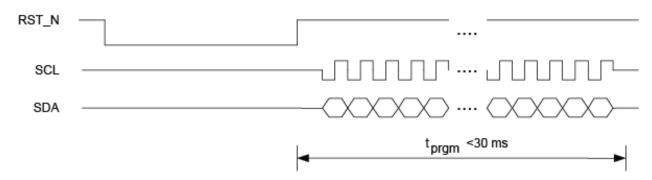
Figure 14. KSZ8895MQX/RQX/FQX/ML EEPROM Configuration Timing Diagram
