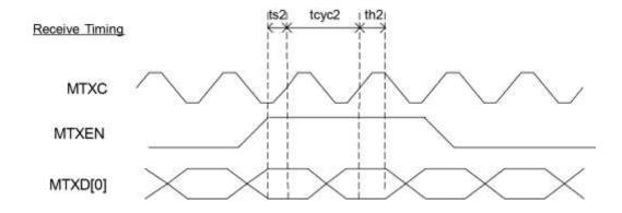
Figure 21. SNI Input Timing
